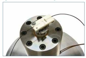
Image 6: Geoshaker with seismic mass
