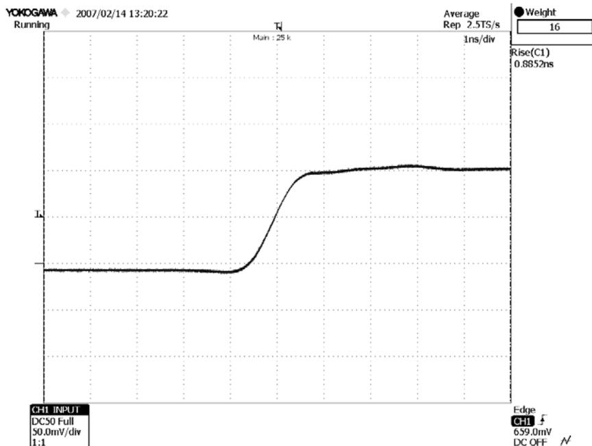
Large Signal Response output signal for 100 MHz, 200  $\mu$ W modulated optical input signal (with 4 times averaging)
