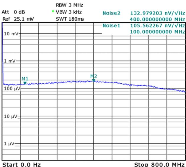
Note: Spectral noise data is measured at the amplifier output with darkened photo diode. To determine the spectral input noise divide the measured output noise by the amplifier conversion gain.
