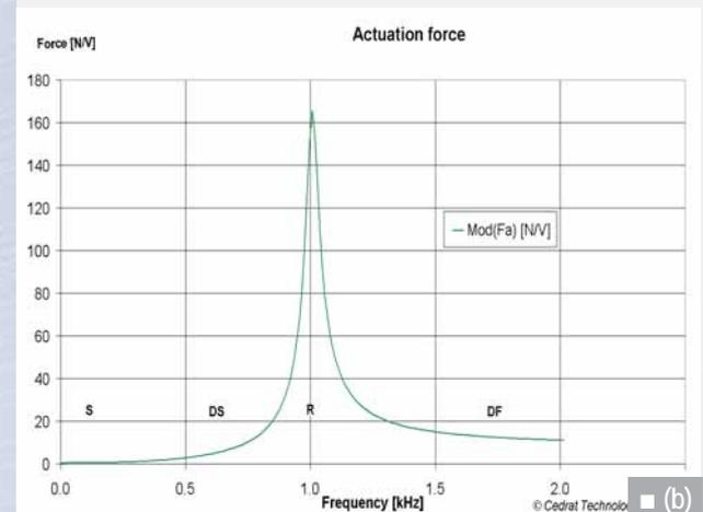
■ Figure 2.19: APA120ML in blocked-free conditions, loaded with a mass of 180gr: Displacement (a) and dynamic force (b) due to inertial forces versus frequency
