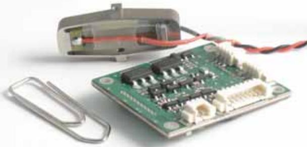
■ Figure 9.1: Evaluation Pack EP120S: APA120S actuator & Cau10 amplifier
