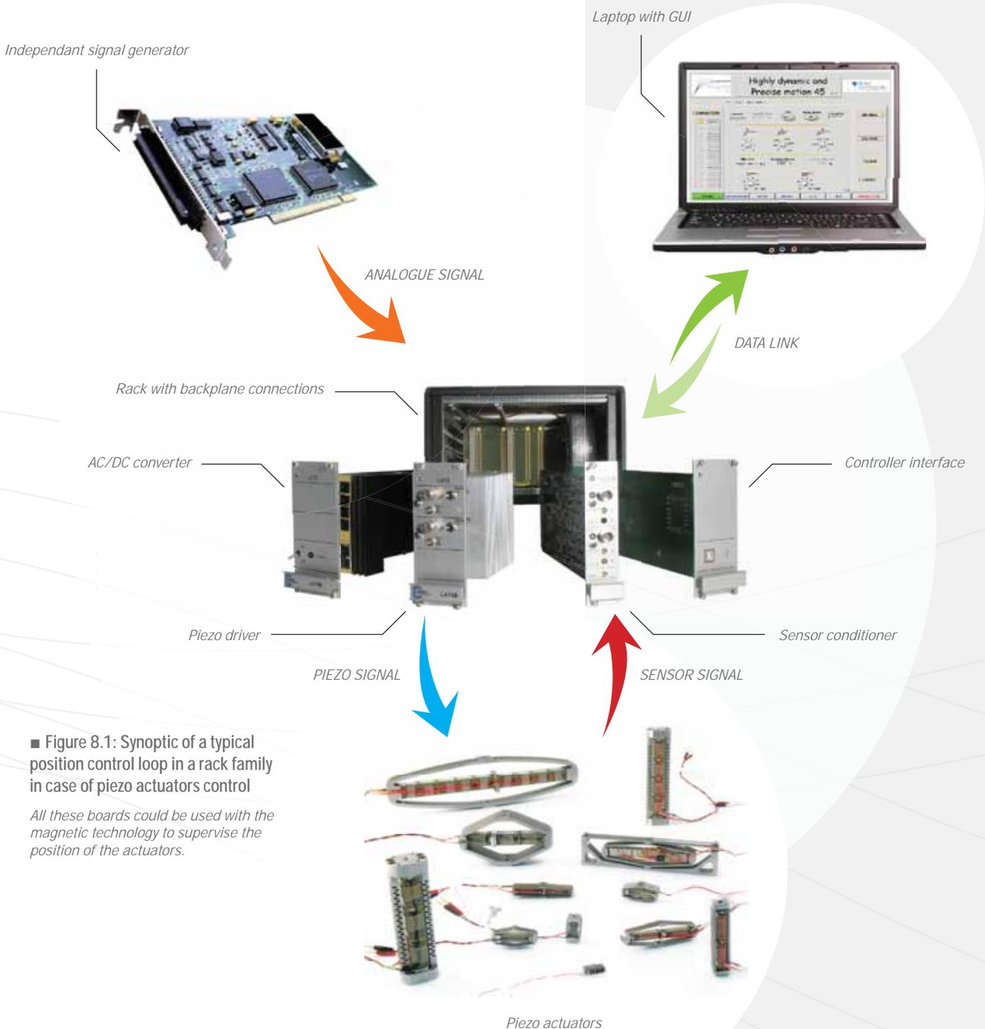
■ Figure 8.1: Synoptic of a typical position control loop in a rack family in case of piezo actuators control
