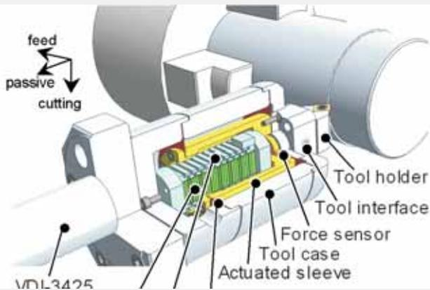
■ Figure 3.9: Smart Tool based on PPA60L (courtesy of IFW)
