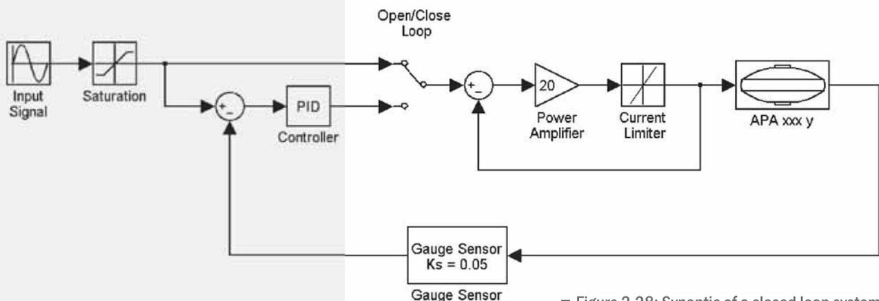
■ Figure 2.28: Synoptic of a closed loop system
