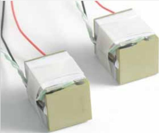
■ Figure 4.1b: Thermocouple sensor on the piezo ceramic
