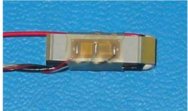
■ Figure 10.1: View of Strain Gauge on an MLA component
