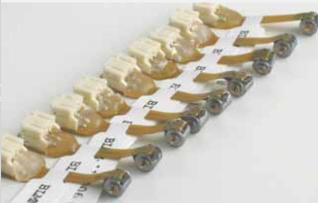
■ Figure 6.3b: A batch of BLMM actuators
