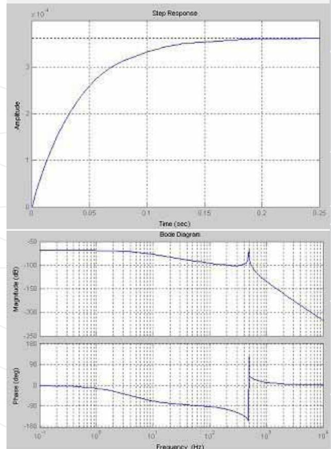
■ Figure 10.7: Closed loop response with stabilizing filters. Step response and Bode response
