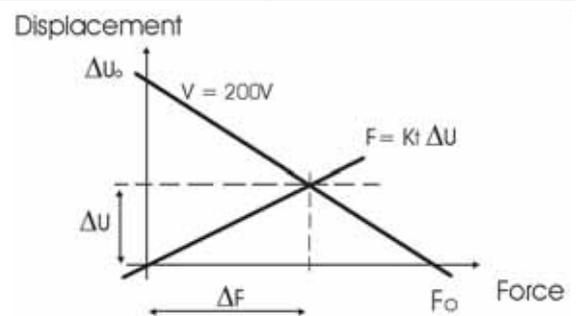
■ Figure 2.13: Load characteristics under a spring with a stiffness  $kt$ .
