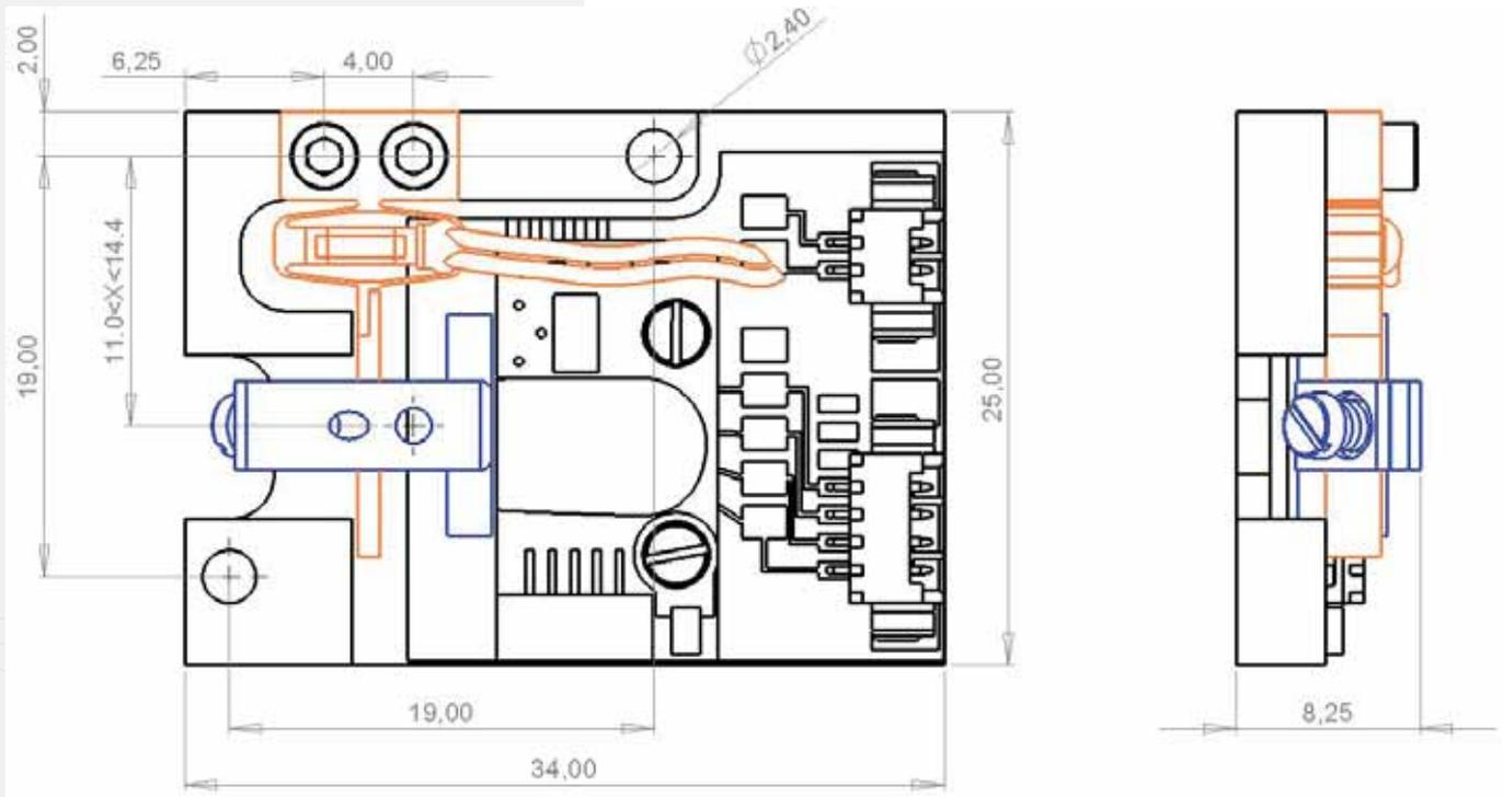
■ Mechanical configuration, with fixed (orange) and mobile part (blue) of the motor
