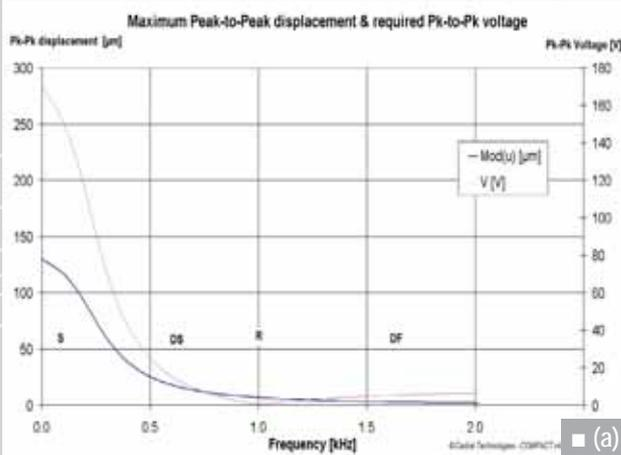
■ Figure 2.21: (a) Modified APA120ML with a low pre-stress (90% less than nominal) under blocked-free conditions, loaded with a mass of 180gr: Maximal displacement and maximal applicable voltage versus frequency.
