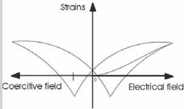
■ Figure 2.18: Electrical field-strain relation in a piezoelectric material
