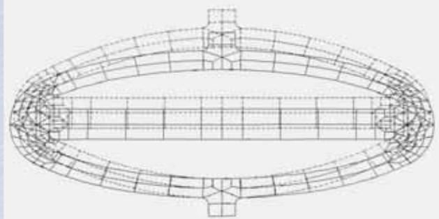
■ Figure 2.8: Finite element computation of an Amplified Piezoelectric Actuator APA®; dotted lines = structure at rest; full lines = structure deformed by the piezoelectric effect (ATILA FEM result).
