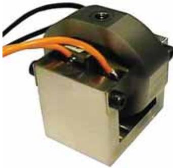
■ Figure 3.13: View of an Ultrasonic Piezo Actuator (UPA)
