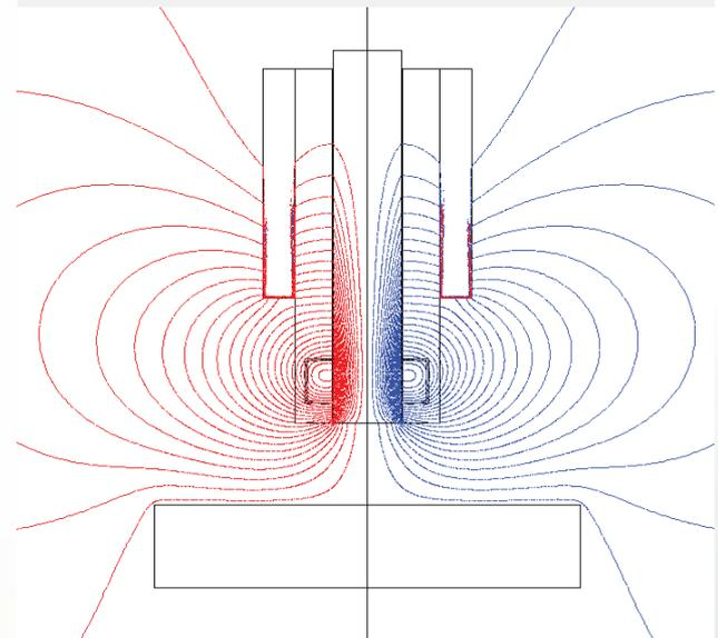
■ Figure 8.3a: Physical principle of an Eddy current sensor probe
