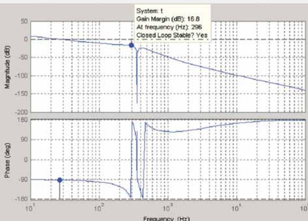
■ Figure 10.5: Open loop response with PID controller and stabilizing filter
