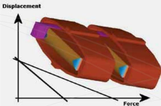
■ Figure 2.14: Series (a) and Parallel (b) arrangements of APA®
