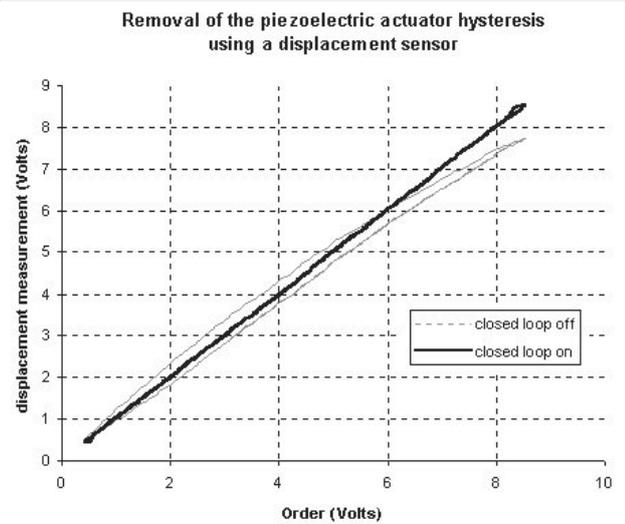
■ Figure 2.29: Example of an hysteresis removal using a SG displacement sensor
