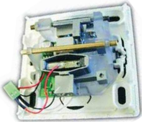
■ Figure 3.17: Piezo generator based on APA60SM, for converting mechanical shocks into electrical power generation (courtesy of LEGRAND)
