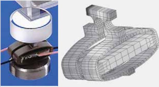
■ Figure 3.3: Tilt-translator TT50S (based on 2 APA50S Actuators) and producing an angular displacement of +/- 0.5° and a resonance frequency of 1800 Hz, a) Actuator; b) corresponding FEM modelling
