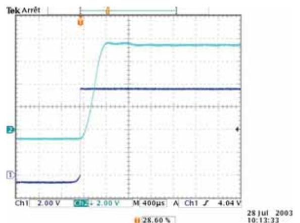
■ Figure 2.31: Mechanical response in closed loop. Channel 2 of a piezo actuator to a step voltage signal (channel 1)
