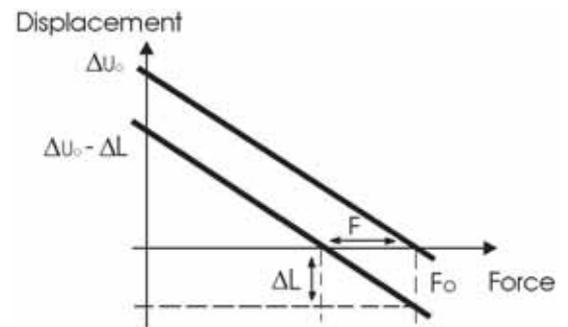
■ Figure 2.12: Position shift and load characteristics of the Actuator under a constant force
