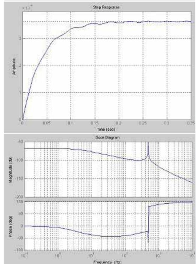
■ Figure 10.6: Closed loop response without stabilizing filters. Step response and Bode response
