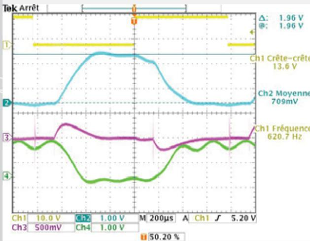
■ Figure 2.24: Temporal excitation and resolution displacement of the APA® during the lifetime test (from top to bottom: Order, Voltage, Current, Displacement)
