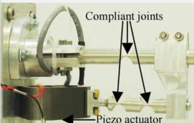
■ Figure 3.10-b: ACV with APA® on Cardiolock medical robot (courtesy of IRCAD)
