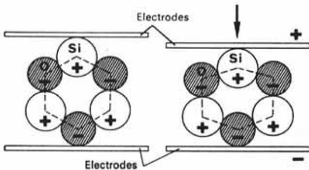
■ Figure 2.2: Piezo effect on the crystal structure (example of the quartz)
