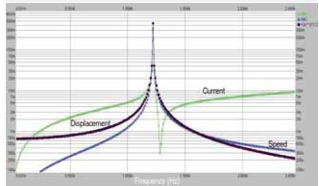
■ Figure 2.15: Current, displacement and speed of the Actuator versus frequency: the resonance effect can either be seen on the Actuator's speed or on the current
