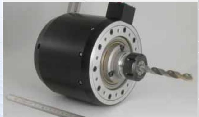
■ Figure 9.8b VTH Vibrating Tool Holder for vibration drilling assistance
