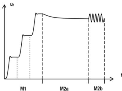
■ Figure 2.10: Example of displacements performed by SPA (M1: long stroke stepping mode, M2a: short stroke quasi-static deformation mode, M2b: dynamic deformation mode)
