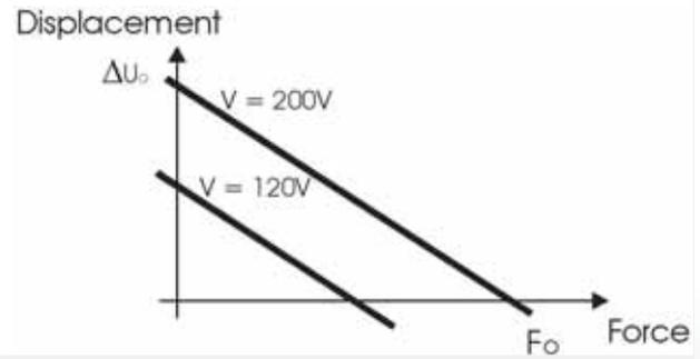
■ Figure 2.11: Load characteristics of a Piezoelectric Actuator
