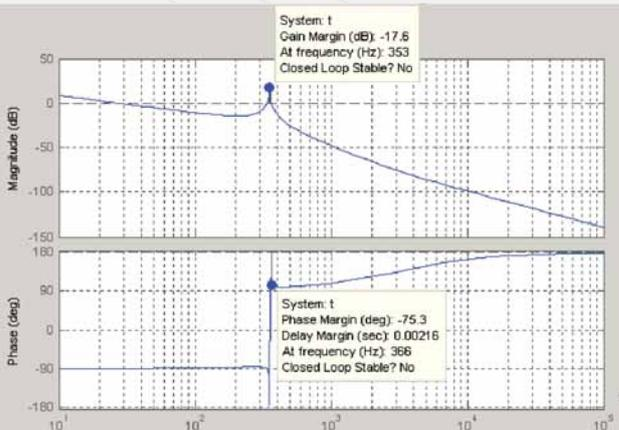
■ Figure 10.4: Open loop response without stabilizing filter
