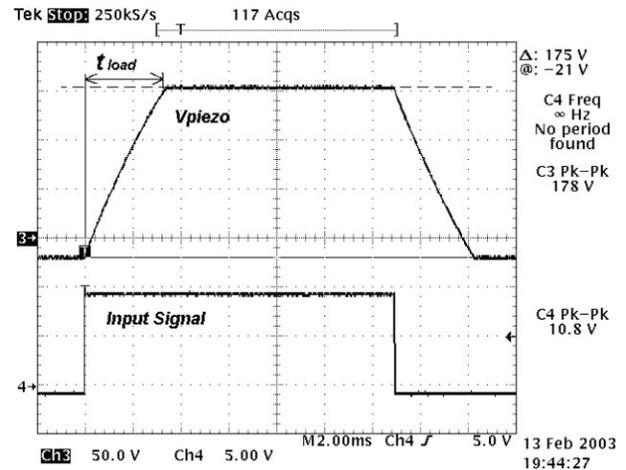
Figure 2.26: The current limitation limits the voltage slew rate of the piezo
