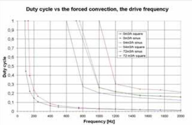
■ Figure 2.23: Limitation of the standard APA-60SM due to the self-heating
