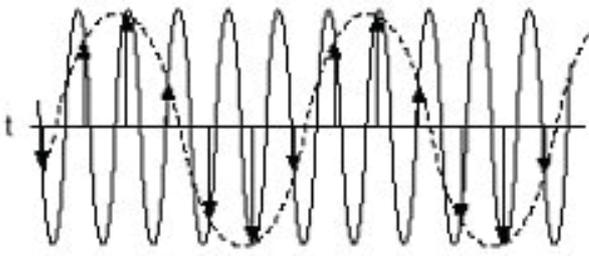
■ Figure 10.9: Example of an Aliased signal: dotted line: Alias recorded by the converter
