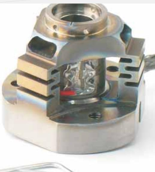
■ Figure 3.19: HPPA for the first European space Lidar, Aladin/Aeolus (courtesy of Galileo Avionica)
