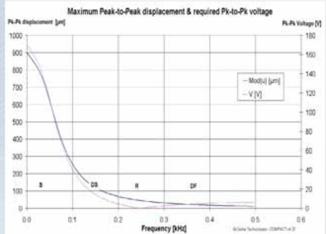
■ Figure 2.22: APA200M and APA900M in blocked-free condition, unloaded: Maximal displacement according to pre-stress and maximal applicable voltage versus frequency.
