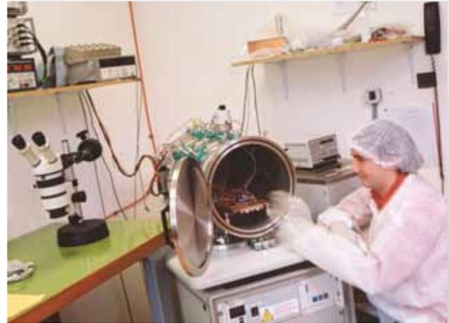
■ Figure 3.28b: View of CEDRAT TECHNOLOGIES labs, thermal Vacuum chamber
