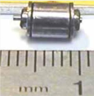
■ Figure 3.25: BLMM Bi-stable Linear Moving Magnet actuator
