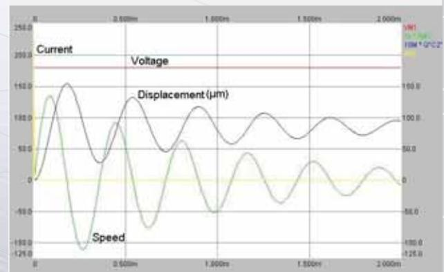
■ Figure 2.17: Step response of the APA60S Actuator
