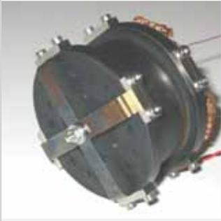
■ Figure 3.22: View of a Voice Coil Actuator usable in Vacuum (3 mm of stroke)
