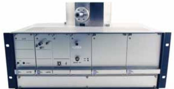
■ Figure 9.8a SPT500L for oval piston machining lying on the associated electronics
