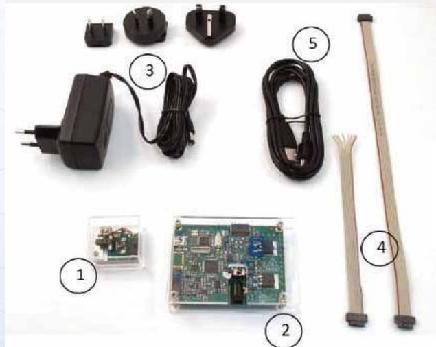
■ Figure 9.6: Components of the LSPA30uXS developer kit
