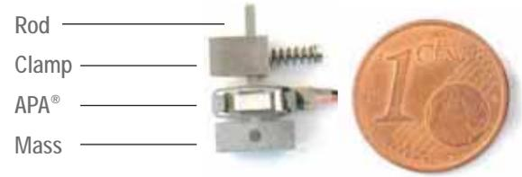
■ Figure 9.5: LSPA30uXS components and principle
