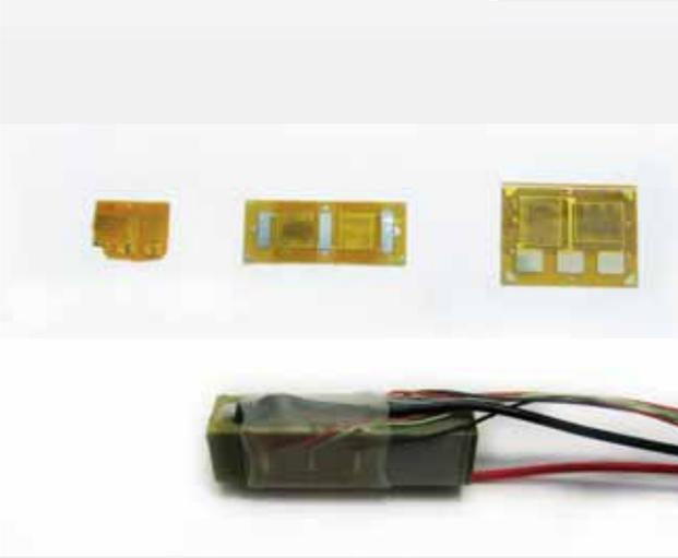
■ Figure 8.2: Strain gages implemented into piezo actuators
