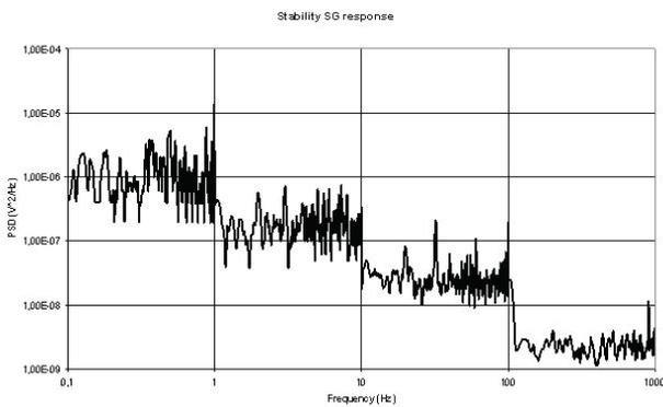
■ Figure 10.3: Cumulated noise of a full SG bridge
