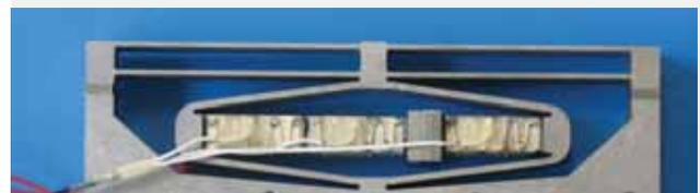
■ Figure 4.2b : Double blades guided Amplified Piezoelectric Actuator APA
