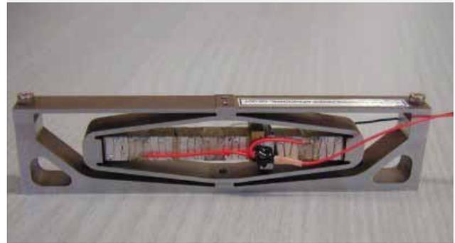
■ Figure 4.2a : Single blade guided Amplified Piezoelectric Actuator APA
