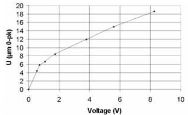
■ Figure 2.16: Relation between the displacement and the voltage for an APA60S at resonance
