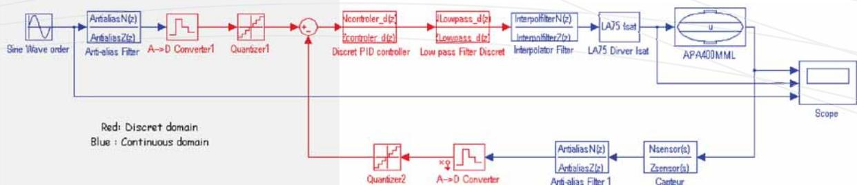
■ Figure 2.32: Schematic of a discrete feedback control loop
