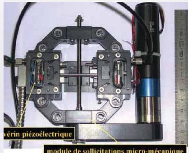
■ Figure 3.11a: Cycling Stress Machine (courtesy of 3S Lab, UJF)
