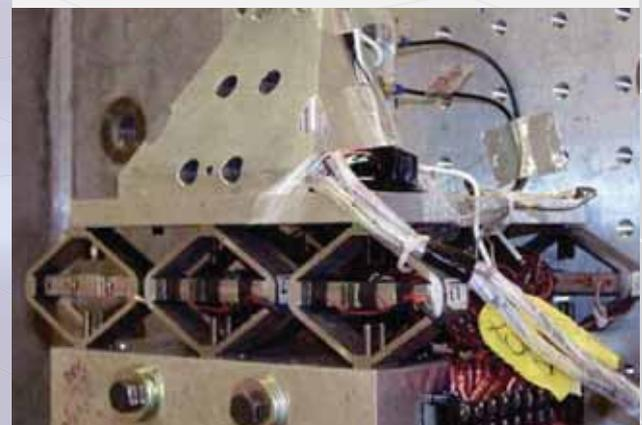
■ Figure 3.12: Piezoelectric shaker (courtesy of Sandia Lab)
