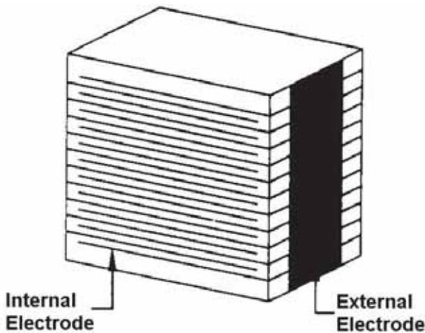
■ Figure 2.1: Schematic view of a MLA
