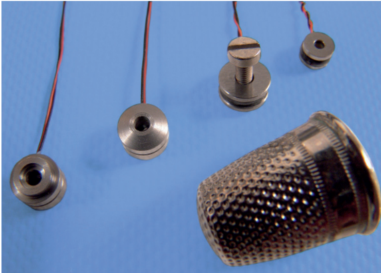
Fig. 4: Set of various types of micro shakers, thimble for comparison of size
