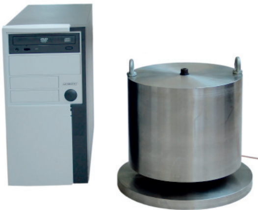
Fig. 2: Geo-shaker for low frequency excitation of soil or buildings (PC case for comparison of size)
