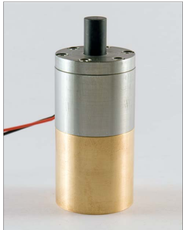
Figure 6b: Single output piezo-shock-generator: brass part: seismic counter mass.
