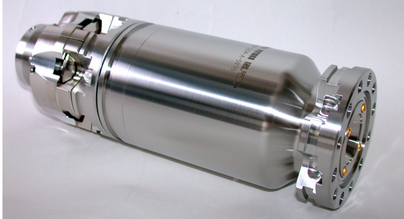
EGF-3104 Electron Flood Gun mounted on a 2¾ inch CFF is rotatable, and has two sets of six mounting bolt holes, one set tapped and one set clear, to allow a user choice when mounting. All high voltage is totally enclosed in the multiconductor triaxial 20 kV cable and metal to metal shell connector.
