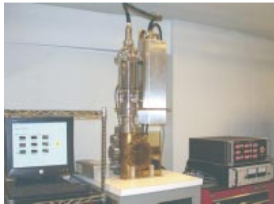
A typical lab set-up of a complete Kimball Physics high energy system with a focusable electron gun, power supplies and optional computer control system (details vary with gun model)
