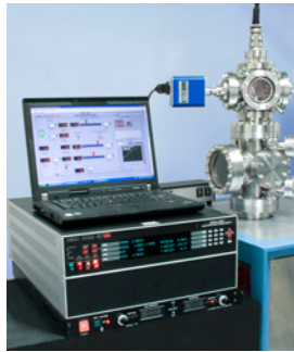
A typical lab set-up of a complete Kimball Physics high energy system with an flood-style electron gun, power supplies and optional computer control system (details vary with gun model)
